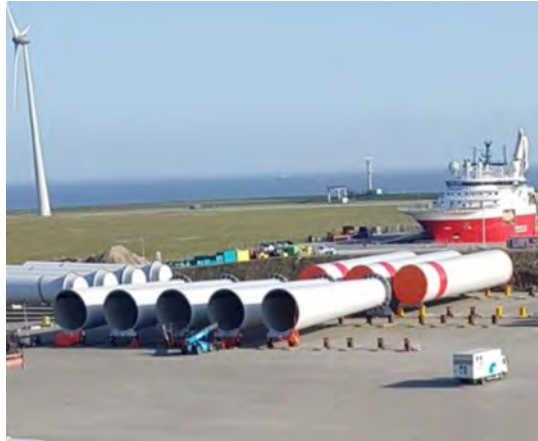
Figure 18 Port Layout example for manufacturing and storage of towers.
