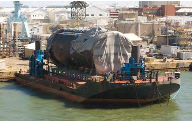
Figure 65 A section of submarine hull being transport by barge
