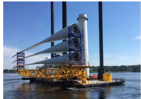
Figure 14 – Blades being transported by jackup barge
