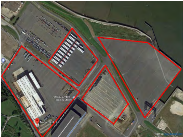
Figure 17 Port layout example for manufacturing and storage of towers.
